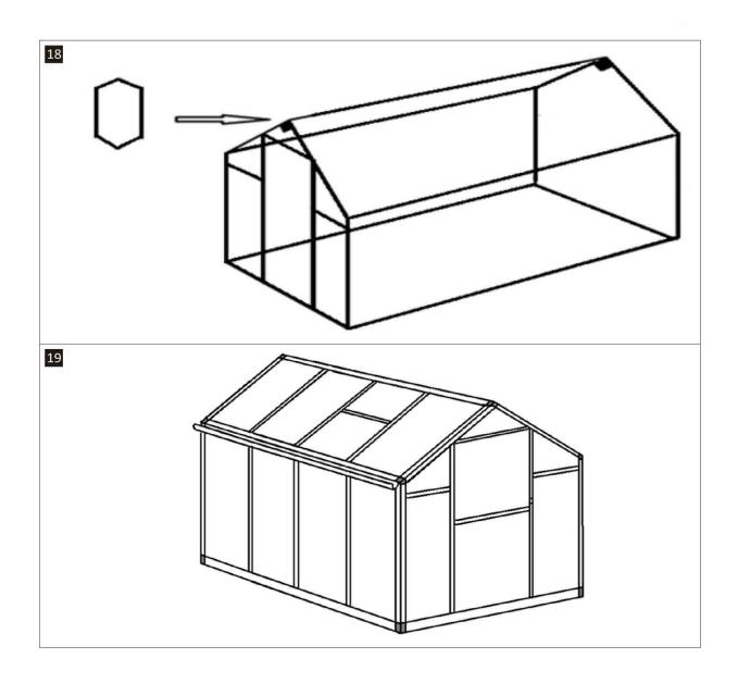
In the end, In order to enhance the fastness of greenhouse, adjust the screws.
