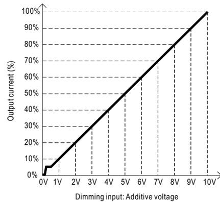
◎ Applying additive 10V PWM signal (frequency range 100Hz ~ 3KHz):
