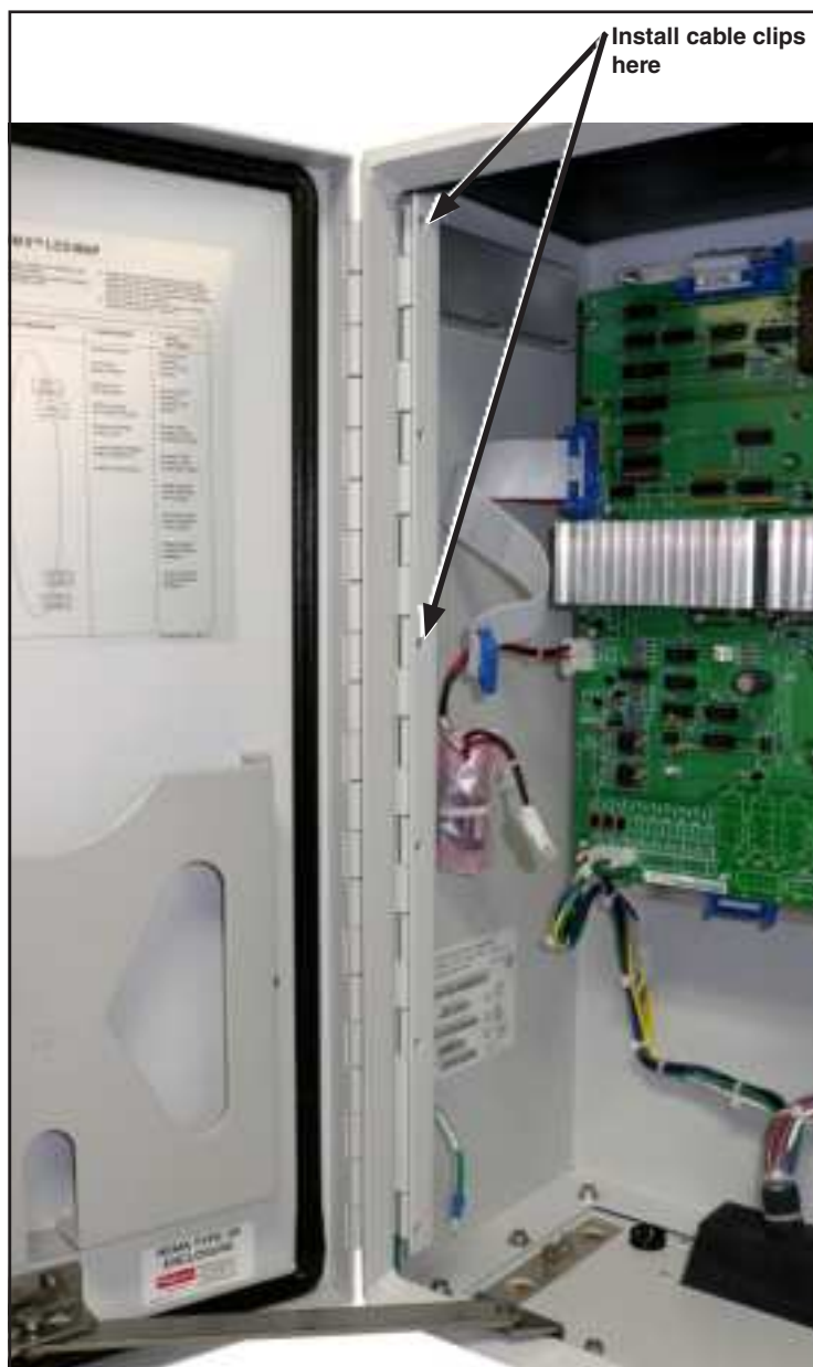
Figure 8. Cable clip locations at the front panel.
