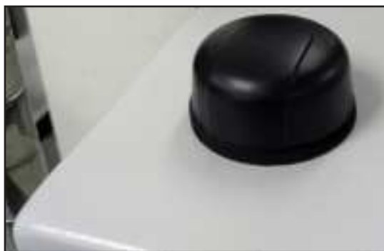
Figure 7. Exterior view of the installed GPS antenna.
