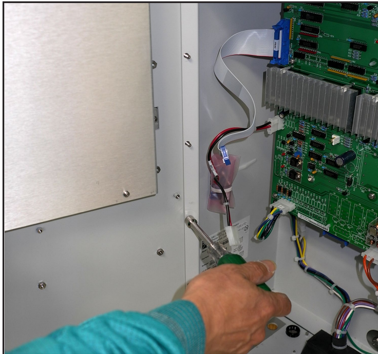
Figure 4. Remove the front panel attachment nuts.
