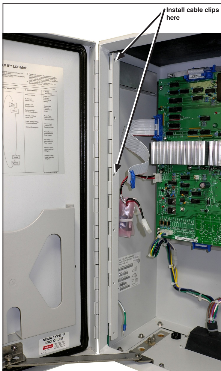
Figure 8. Cable clip locations at the front panel.
