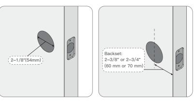
Measure to confirm that the hole in the door is 2-1/8" (54mm). Measure to confirm that the backset is either 2–3/8" or 2–3/4" (60 or 70mm).
