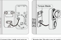
Rotate the Thumb turn in vertical position and insert the horizontal orientation of torque blade into the interior assembly lock switch.
