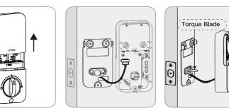
Remove the battery cover. Connect the cable and ensure tight cable connection.
