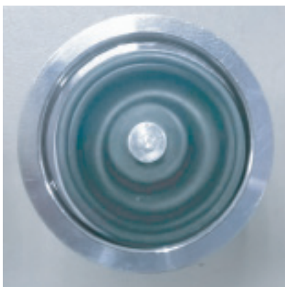
Figure 9 - Correct diaphragm alignment
