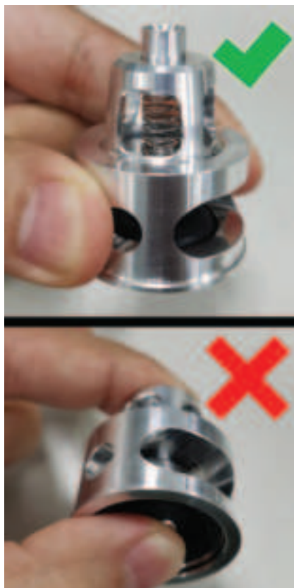
Figure 12 - Proper handling of the diaphragm.
