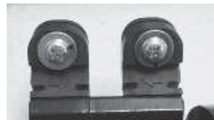
Figure 171 - Water pump gasket boot orientation
