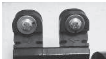
Figure 187 - Water pump gasket boot orientation
