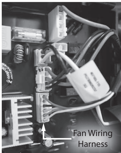
Figure 95 - Locate fan wiring harness on control board
