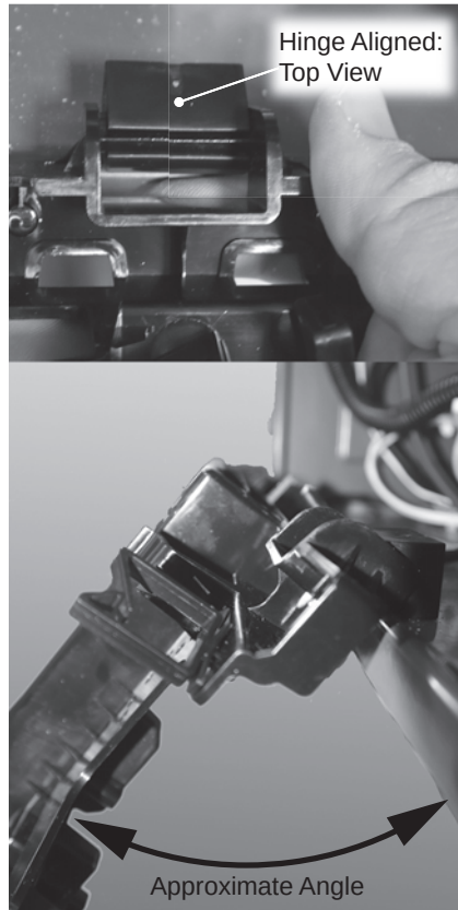
Figure 26 - Removing the control board.
