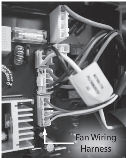
Figure 110 - Locate fan wiring harness on control board
