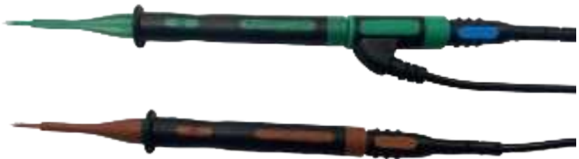
Fig 3. Prods in 2 wire testing configuration
