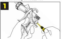
Turn the Fluid Adjustment Knob(D) counterclockwise to remove Fluid Needle and Needle Spring.
