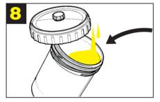
Mix coating material by Manufacturers' instructions and pour into the Paint Cup,
