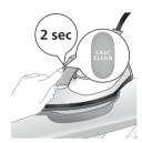
7 Press and hold the CALC-CLEAN button for 2 seconds until you hear short beeps.
