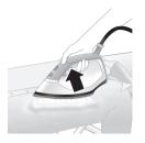
7 Press and hold the steam trigger to start ironing.
