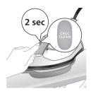
8 Press and hold the CALC-CLEAN button for 2 seconds until you hear short beeps.
