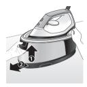
${f 3}$  Press the lever in the water tank handle and remove the water tank from the base.
