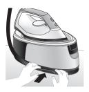
3 Fold the supply hose and wind the supply hose inside the supply hose storage compartment.
