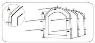
**STEP-2**:Place the remaining five short support rods (B) on the side of the carport, and the Curved support rod and Side support rod are assembled as shown at point A
