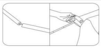
**STEP-1:**Connect the support rods and thread them through one end of the bicycle shed fabric, and do the same on the other side
