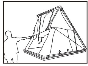
2. The elastic helps keep the tent inside the housing. Slide the elastic strap down and place it around the tent base when setting up.
