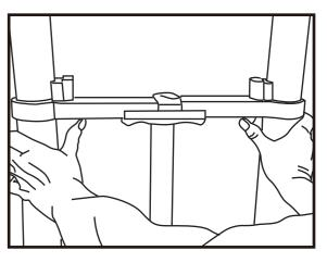
3. To close the ladder, grasp with both hands and press the left and right switches on the lowest cross piece. Slowly collapse the ladder in the opposite sequence to opening it.
