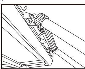
Take the ladder out from the storage bag and remove the strap that is holding the retracted ladder in place. Clamp the ladder onto the brackets on the rooftop tent extending each rung sequentially. Before attempting to extending the next rung pull each rung to its full extension and ensure that the locking mechanism is engaged.
