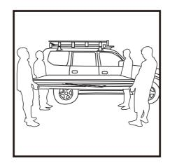
1. With no less than four people, lift the rooftop tent onto the roof platform. Make sure the main door is facing backwards from the vehicle before attempting the lift. Centre the tent ensuring the weight is distributed evenly. Ensure the rear of the tent is flush with the vehicle so the ladder can be fitted.
