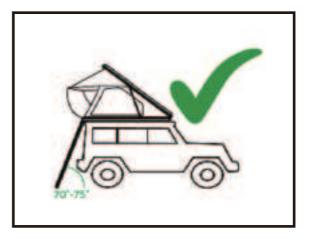
Adjust the length of the ladder to make sure the angle is approximately 75 degrees between the ladder and the ground.
