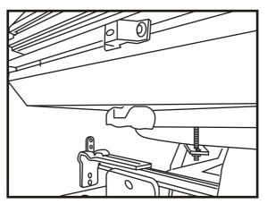
3. Insert the optional end caps to the end of the extrusions.
