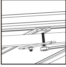
Secure each of the four corners with the brackets and screws provided. Each mounting point requires two 55mm M8 screws that slide into the slots on the mounting bar. Tighten the Nyloc with washer using the spanner provided.
