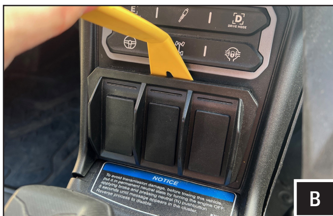
B. Remove the rocker switch panel using a plastic pry tool.
