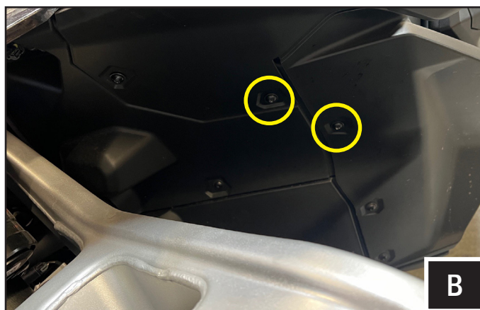
B. Remove the (2) factory T-30 screws, circled above, on the driver side wheel well liner.
