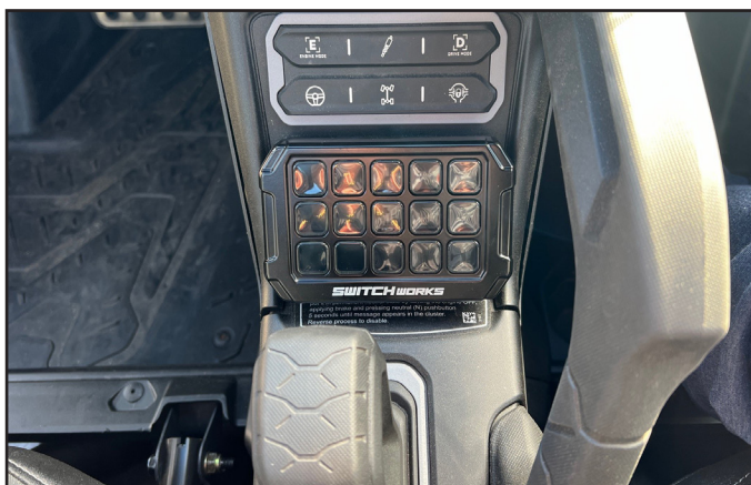
Completed installation of 15-Button Controller.
