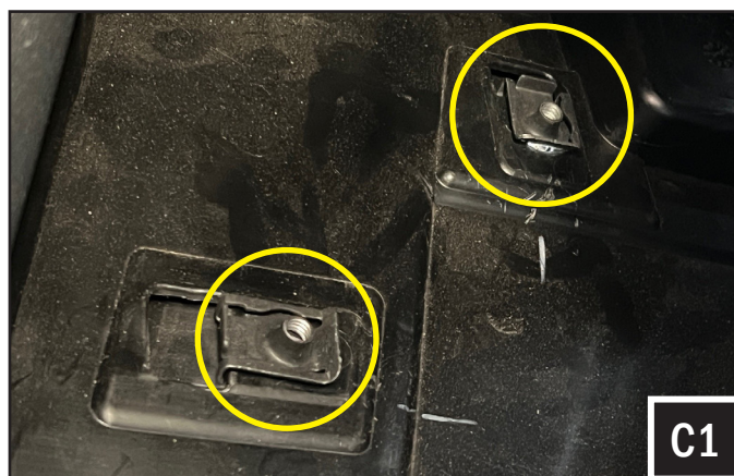
C. It might be easier to remove the (2) U-Nuts from inside the vehicle.
