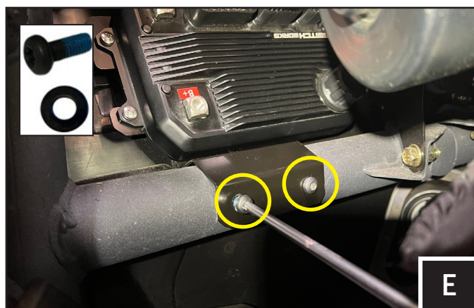
E. Use the (2) M6-16mm screws and washers [B-HPM616-2], included in the kit, to secure the Mav R brain bracket to the factory PEM nuts in the tubing.
