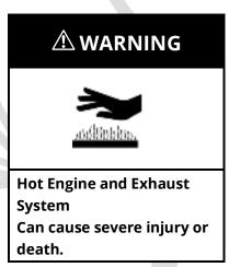
During operation, some parts of the generator set can become extremely hot. To avoid burns, allow the engine to cool sufficiently before changing the coolant. DO NOT remove the radiator cap while the radiator is hot. Doing so could result in extremely hot coolant spraying out. Severe burns may result.
