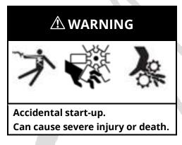
**WARNING:** Putting the generator set in AUTO mode may cause the generator set to start without warning. This can result in severe injury or death.
