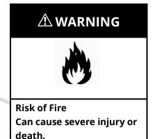
During operation, some parts of the generator set can become extremely hot. To avoid burns, allow the engine to cool sufficiently before bleeding the fuel system.
