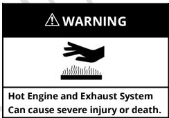
During operation, some parts of the generator set can become extremely hot. To avoid burns, allow the engine to cool sufficiently before checking the engine oil.
