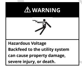
Whenever the generator set is connected as standby power, a transfer switch is required to prevent electrical backfeed into the utility electrical grid. Electrical backfeed is illegal and can result in the severe injury or death of utility company personnel working on power lines. The generator set must be installed following local, state, and National Electric Code (NEC) guidelines.
