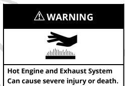
During operation, some parts of the generator set can become extremely hot. To avoid burns, allow the engine to cool sufficiently before changing the intake air filter.
