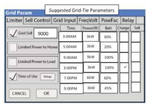
Note: Change the programming from Percentage to Voltage in the Battery setup menu. (Use Batt % Charge / Use Batt V charge)
