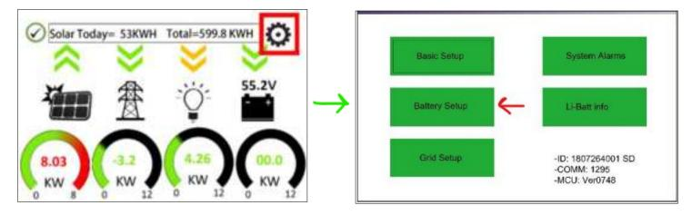
**2.** Program the 'Batt' tab first. Enter the settings as shown below and tap on 'OK' in the bottom of the menu afterwards:
