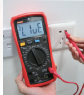
Live and nature wires identification
