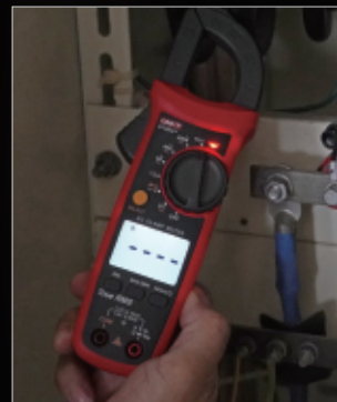
NCV multi-segment display and audio/visual alarm
