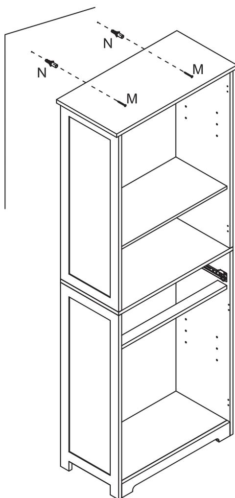
**EN** If it is a solid wall, please use expansion and self-tapping screws, if it is a wooden wall, only use self-tapping screws, please do not overtighten the screws
