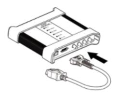
Figure 5-1 VCMI Connecting to Main Cable V2.0
