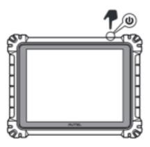
Figure 6-16 Power up the Tablet
