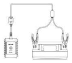
Figure 13-4 Battery Tester Connection Example 2
