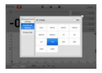
Figure 11-76 Amplitude Setting Screen (DC 10 V)
