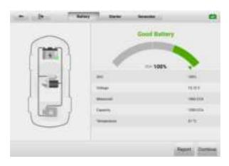
Figure 13-7 Battery Test Results Screen
