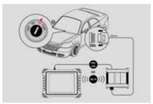
Figure 11-107 Connection Diagram
