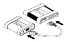
Figure 6-2 VCMI Connecting to EVDiag Box
