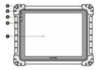
Figure 2-1 MaxiSys Tablet Front View
