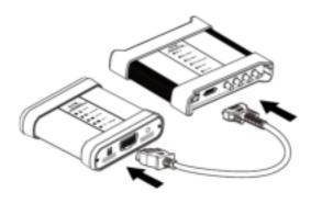
Figure 5-2 VCMI Connecting to EVDiag Box
