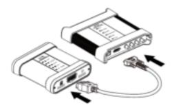
Figure 6-15 VCMI Connecting to EVDiag Box
