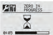
Figure 44. Zero Calibration in Progress
