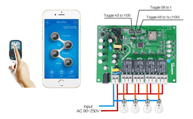
2. In inching mode, you can turn on the connected devices for 1-16s . For example, you can turn on CH1 connected device for 1s, then auto-off.
