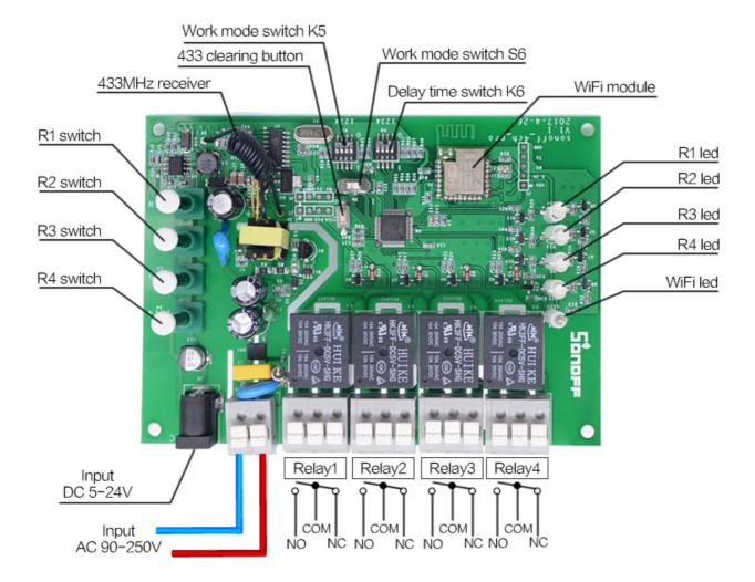
You may choose to power up by 5-24V DC or by 90-250V AC. Each relay without voltage output.
