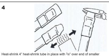
Heat-shrink 4" heat-shrink tube in place with 3/8" over end of smaller heat-shrink tube. Remove heat, resqueeze at end of smaller heat-shrink tube, then squeeze at end of outer heat-shrink tube. Hold for 10 to15 seconds.
