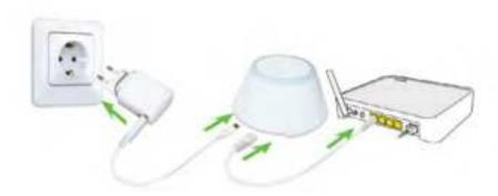
To begin the pairing process the Gateway should be plugged into the power supply and connected to the Internet. Also, make sure that the UGE600 is added to your Salus Smart Home App. For the installation of the Universal Gateway, please refer to the UGE600 manual on salus-manuals.com
