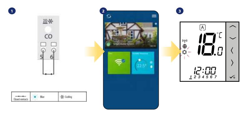
When there is jumper at "CO" terminal KLO8RF is automatically working in cooling mode.
