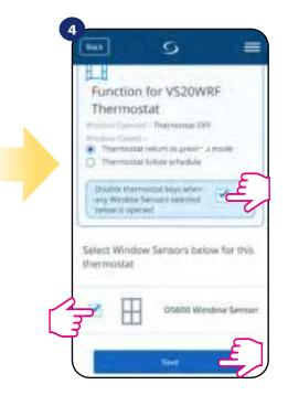
Mark sensors which you want to link together with the thermostat. You can additionaly lock buttons on thermostat when window is opened by marking option above.
