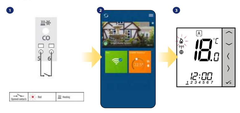
When there is no jumper at "CO" terminal KL08RF is automatically working in heating mode.
