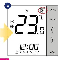
Also on the thermostat's display you can see that frost protection mode is activated by "Snow" icon.
