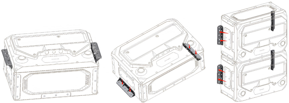
Figure 3: HUSKY 2 Mounting Installation
