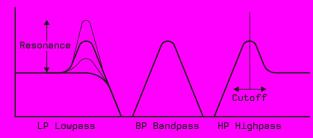
The HP/BP/LP switch selects the filter type. HP=Highpass: passes frequencies above cutoff (cuts bass)
