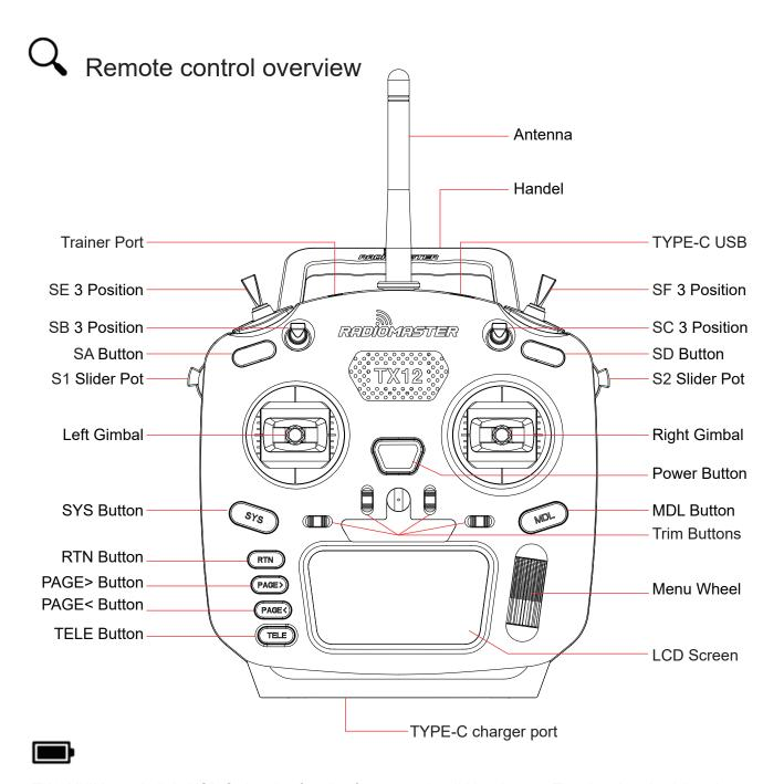
TX12MKII has a built-in USB-C charging function for 3.7v to 4.2v lithium battery. The charging circuit is only suitable for 2x 3.7v Li-ion 18650 or 2x 3.7v Lipoly batteries (2s 7.4v Lipo battery pack), the nominal battery voltage is 3.7v, and the maximum charging voltage is 4.2v.
