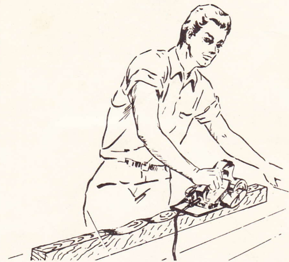
Cut resulting from improperly aligned base
