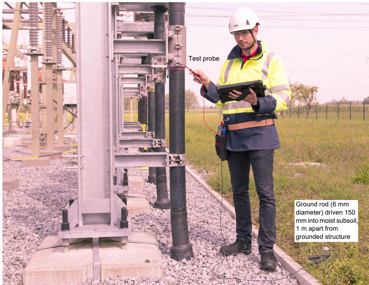
Figure 5-26: Touch voltage measurement with PTM (tablet) according to IEEE 81
