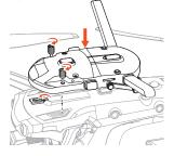
Loosen side brackets, rotate to diagram position, and tighten clockwise into fuselage screw holes.
