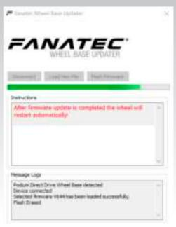
When the update is done the Podium Wheel Base DD1 will restart automatically after firmware update is completely finished (shown right):
