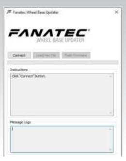
When the Wheel Base Updater is connected to the Podium Wheel Base DD1 the buttons 'Load Hex File' and 'Flash Firmware' are available (shown right).
