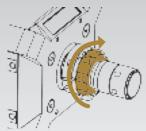
Position the locking ring until it touches the rubber gasket, but do not tighten. This keeps the rubber gasket in place during wheel rim attachment.
