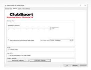
The bar Wheel angle / sensitivity can adjust the maximum turning angle of the Podium Wheel Base DD1, so the functionality is identical with the option 'SEN' in Tuning Menu (see chapter 'Tuning Menu' of this manual for more detailed information). Please note that in Tuning Menu the value for 'SEN' must be set to 'AUTO' to allow the PC driver to take the control. If in Tuning Menu 'SEN' is set to any other value than 'AUTO' this value is applied and the PC driver has no influence.
