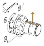
Centre the DD1's Quick Release shaft so that the slot is facing up.
