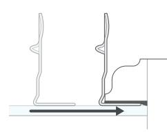
Locate the correct position for the brackets by holding a credit card or store card vertically in the corner of the glass - the bracket will sit in line with the edge of the card.
