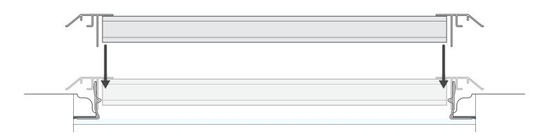
Push the frame towards the window until the oval slots lock onto the prongs of each of the brackets. The installation of the blind is now complete.
