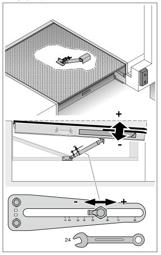
▶ Loosen the sensor. Shift the sensor in the holder.
