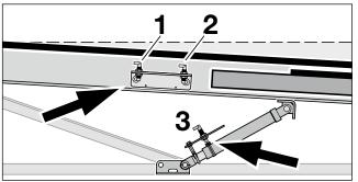
The sensor holder for sensor 1 and 2 must be at the bottom of the platform beam.
