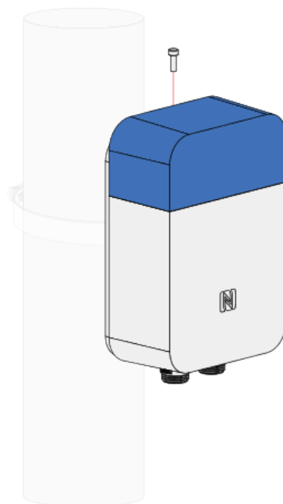
Figure 12: Fasten the device and the bracket
