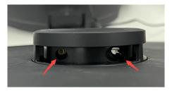
Please manually press the radar cover to ensure it springs back normally. Also, press and hold the radar cover to check if the robot vacuum cleaner consistently moves backward.
