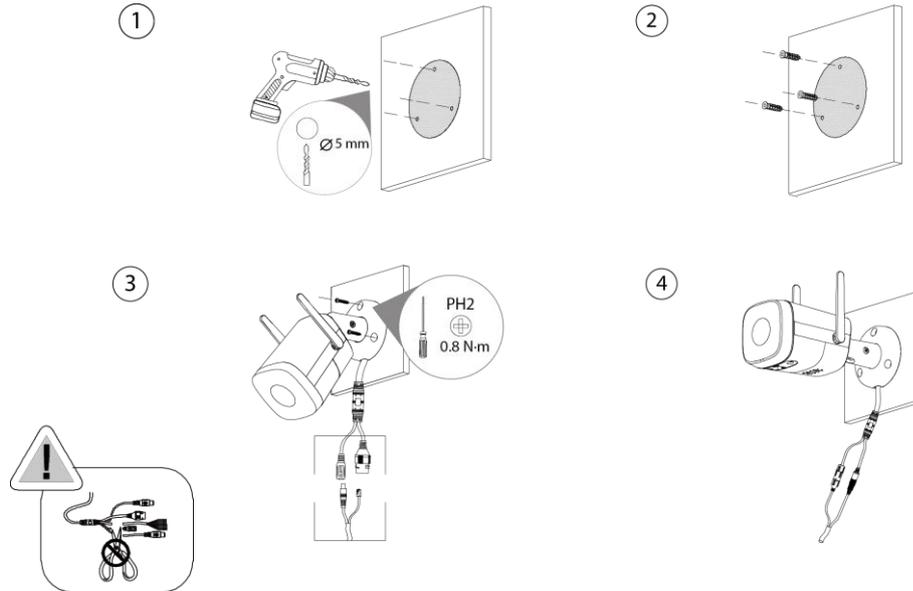
Figure 4-6 Cable going through the mounting surface
