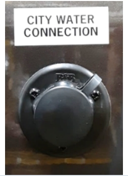
City Water Fill w/Connection Label
