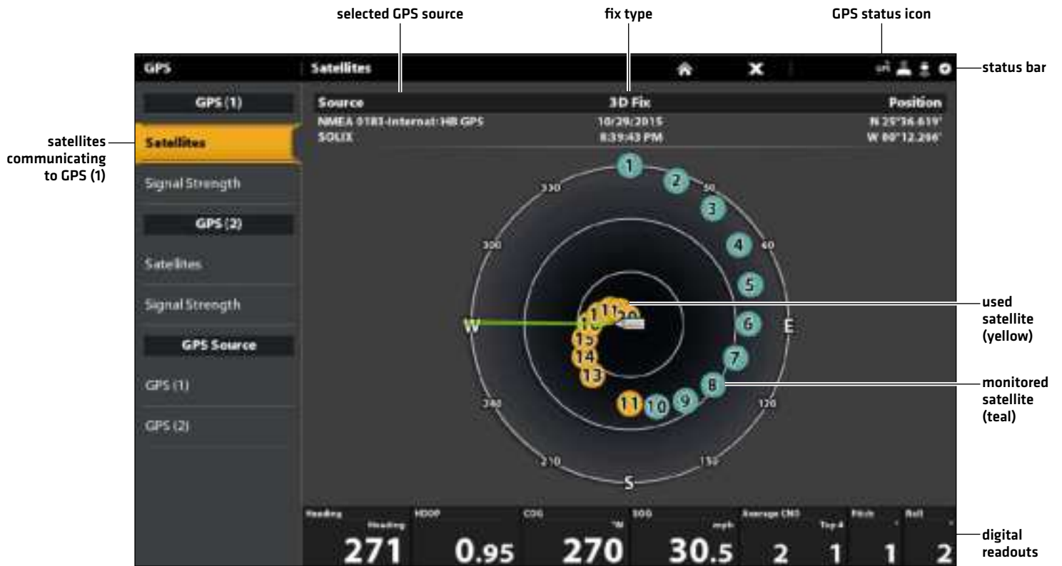
GPS (1) Satellites shows a sky chart and numerical data from the selected GPS receiver
