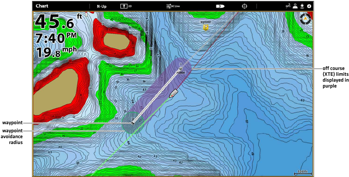
Chart View with Alarm Overlays Displayed [Humminbird LakeMaster]
