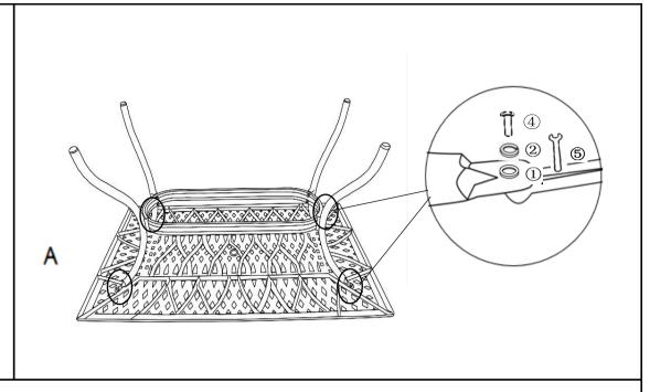
Lay the Table Top(A), top facedown, onto a flat, soft, clean surface. Attach the Table Legs(B) to the Table Top(A) using Washers(①), Spring Washers(②) and Hex Bolts(④) with the Spanner(⑤). At this stage, only loosely tighten the Bolts.
