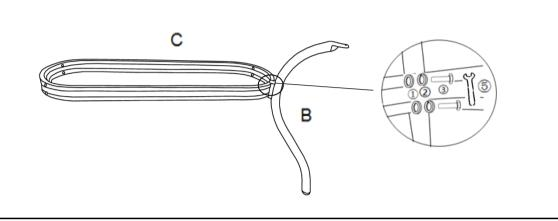
Loosely attach the Central Support Ring(C) to Table Legs(B) using washers(1), Spring Washer(2), and Hex Bolts(3), with the Spanner(5).
