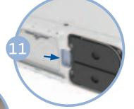
Push the column assembly into the device such that the columns are fully seated into the Inogen One® G5/Rove 6 concentrator. The spring loaded latch button should fully return to the closed position.
