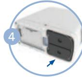
Place the Inogen One® G5/Rove 6 concentrator on its side so that the underside is visible. The metal column assembly can be seen on one side of the device.
