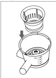
Put the 2 juice screen into the 3 juice container ensuring the dot on the 2 juice screen is aligned with the dot on the 3 juice container.
