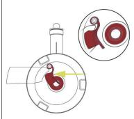
Firmly insert the compression silicone into the slot below 4 the pulp outlet. This silicon is to offer a slop to let pulp goes out. And it makes 4 the pulp outlet can be cleaned easier. Please make sure it is firmly inserted in case of any leak.
