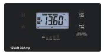
Press and hold the **BATT. TYPE button** for 3 seconds to enter battery type selection mode. The selected battery type will be shown on the LCD meter. The default setting is LFP Battery, and the controller will automatically memorize your selection.
