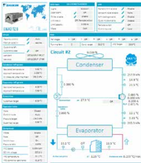
Circuit overview – real-time data For maintenance check and diagnostics.
