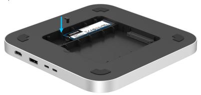
4) Put the Enclosure cover on and fix it in the holes with screws
