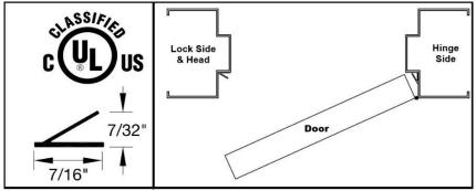
Positive Pressure Tested Gasketing Materials for Fire Doors. Intended for Applicationto/ with listed steel frames and/or classified steel covered composite, hollow metal type fire doors rated up to 3 hours, wood and plastic covered composite type fire doors rated up to 1-1/2 hours, and wood core type fire doors rated up to 20 minutes. Meets UL10B, UL10C and CAN4-S104-2010 Category J .17L5 9903
