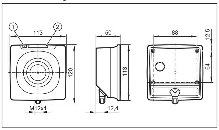
The max. tightening torque of the screws when mounting the device is 0.8 Nm.
