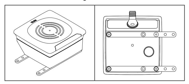
► Fix the device with fixing screws to the designated location.
