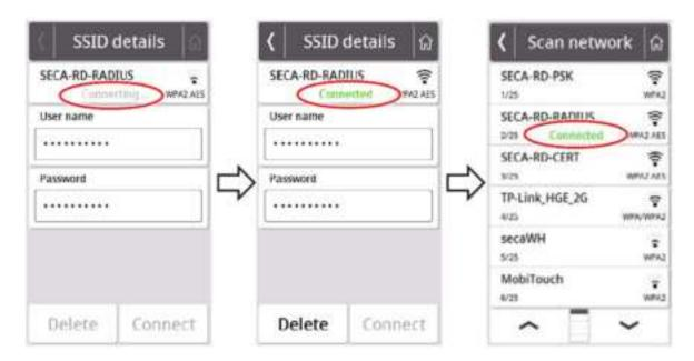
The seca device now establishes a connection to the selected WiFi network. As soon as the connection is established, it will be indicated by the message "Connected" behind the selected network.
