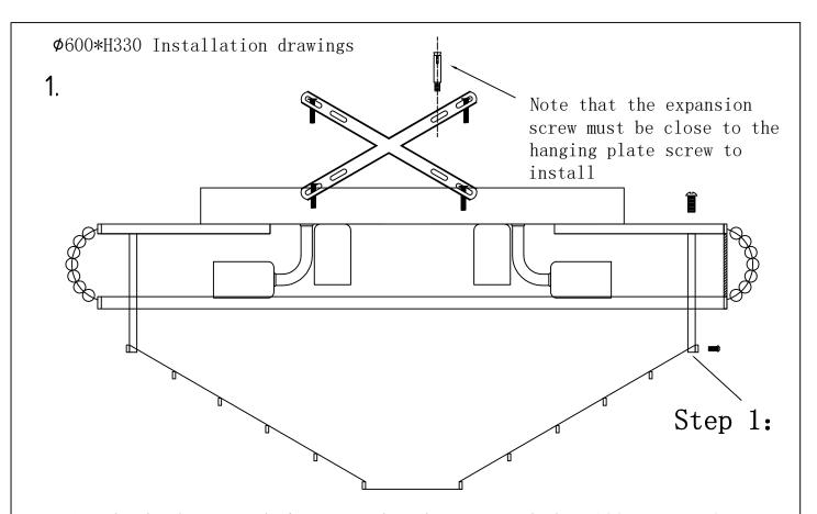
1.Lock the bottom shelf onto the chassis with 6 x 100 square 4 pcs 2.After testing the electricity, the hanging board with expansion screws to the ceiling, and then the lamp body installed on the hanging board
