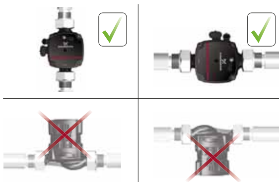
Fig. 4 Pump positions
