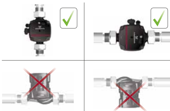
Fig. 4 Pump positions
