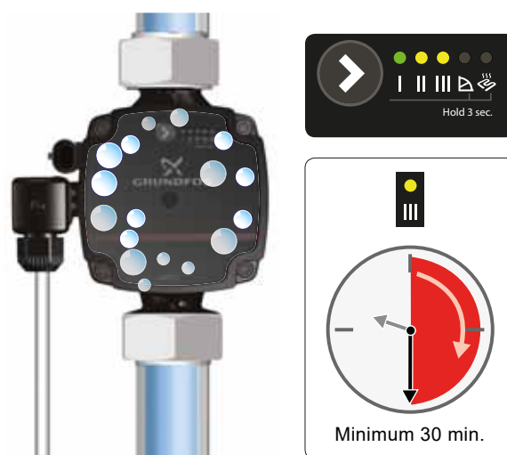
Fig. 7 Venting the pump
